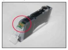
Carefully remove the original chips from original cartridges as the picture shows.
